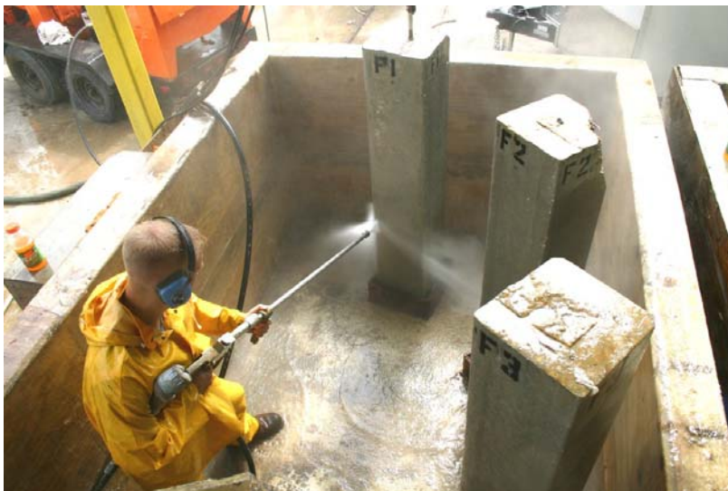
Figure 5.6 Pressure washing test piles with 68.9 MPa water pressure.
